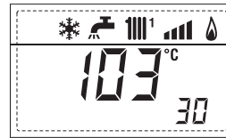
28. Visualisation solar probe temperature value S1 with solar board INSOL
