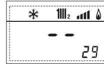
30. Visualisation solar probe temperature value S1 with solar board INSOL
